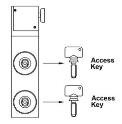
Actuator is locked Both keys are removed
