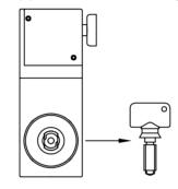
Actuator is locked The key is removed
