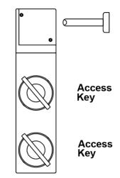
Actuator is released Both keys are trapped
