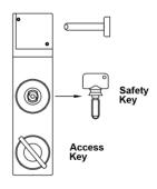
Insert and trap access key into release safety key, the actuator is released
