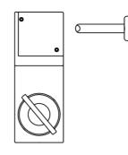
Actuator is released The key is trapped
