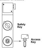
Insert the actuator, insert and trap the safety key the access key is released
