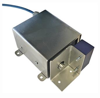
The Mechan stainless steel PLU2 Air operated Locking unit is a complete, fail-safe system designed to lock a Gate or Access Lid securely until it is safe to enter. This can be determined either by a Motion Stop detector or a simple timer. It incorporates both a Bolt Position Sensor Switch and a Mechan Guard switch to sense when the locking bracket is in position. The bolt must be in the out position and the locking bracket in place before the machine can be re-started.
