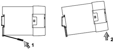
To remove the modules, gently lever out the DIN clip with a small screwdriver as shown (1).
