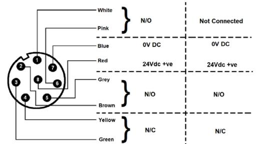
**CONTACT OPERATION** - The N/O contact(s) on Mechan safety switches are open when the actuator is away from the switch. When the actuator is within the specified operation distance, the N/O contact(s) will close and N/C contact will open.
