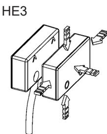
The Targets must be aligned i.e. the arrows together at the top of the switch.
