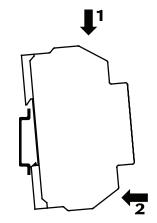
To remove the modules, gently lever out the DIN clip with a small screwdriver as shown (1).
