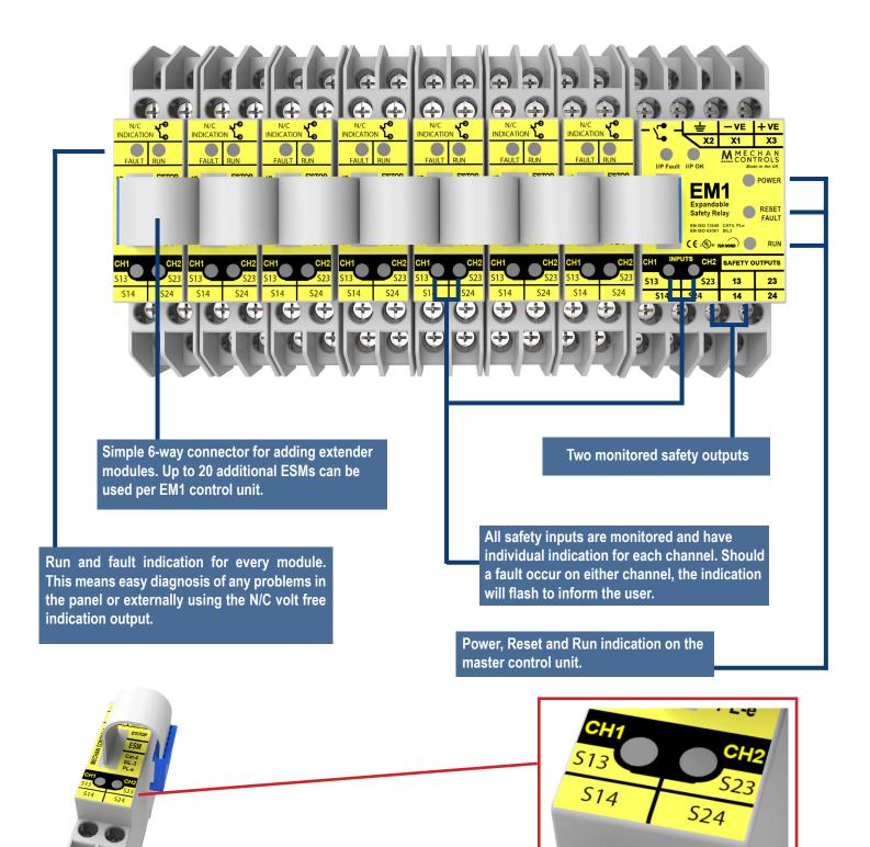
New and improved safety input indication diagnostics. When a channel is faulty, it will now indicate which one by flashing.
