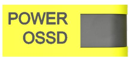
Displays the status of the OSSD outputs and the power supply.
